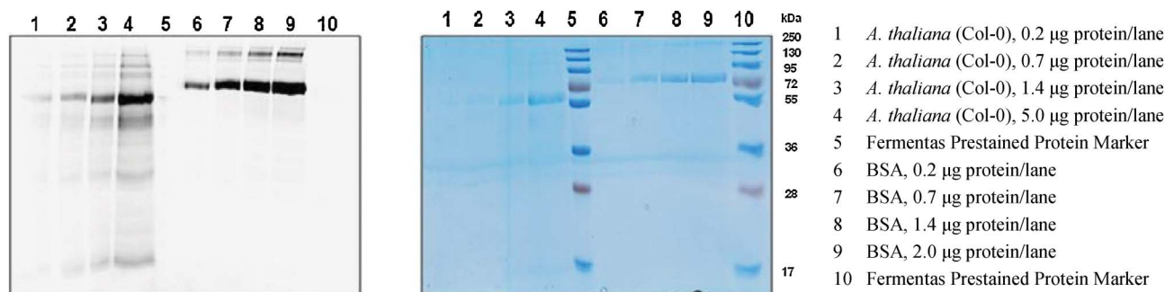
Fig. 3 SDS-PAGE gel of labelled BSA and a crude protein mixture ( A. thaliana (Col-0)), visualised by in-gel fluorescence-scanning (left) or via Coomassie-staining (right).
